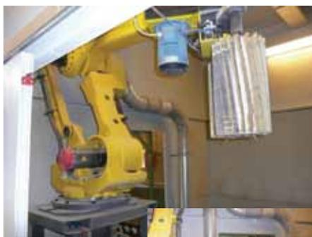
A Flex Trim 3D brush sanding robot (up to six axis) on a high capacity production line in Denmark.
