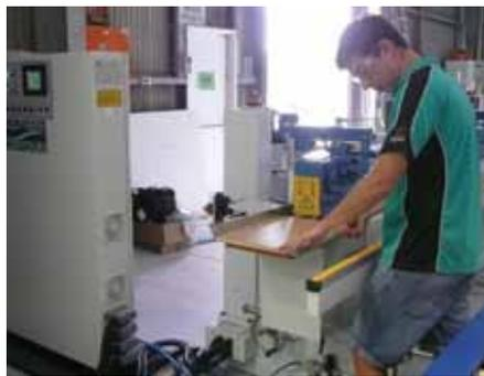
Allen Gray with a programmable seven head Southern Contours edge sander with controlled feed and sanding pressure. The custom built head selection allows greater scope for perfection and productivity improvements.
