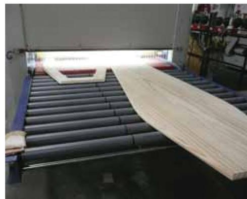
Left & top right: Profiled components being smooth sanded in four directions through a six head Unisander.
