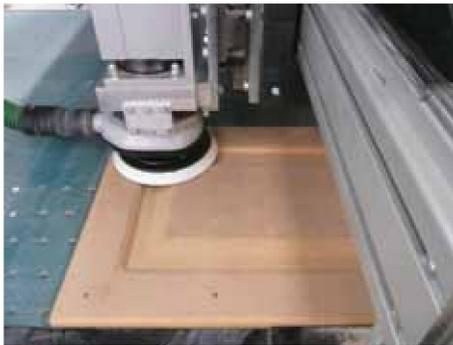
Automated calibration orbital sanding with a Gottschild sander, which also has automated panel size recognition.
