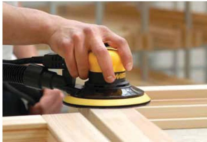
Dust free surface calibration orbital sanding with a Mirka Ceros compact electric sander
