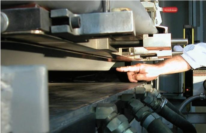
A programmable extra step is now available in the recipe called "One Touch" shown with heater lowered creating a flat membrane. When in cycle with a closed chamber, the foil is also held against the flat surface with vacuum until making contact with the work surface.
