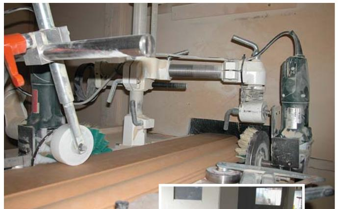
The two discs at work on the edges of the moulding.
