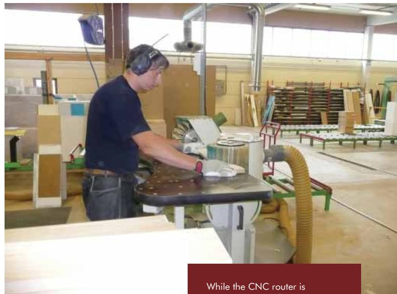
While the CNC router is precision cutting the next components, the manual Flex 100 brush sander is being used to edge sand the previous components by a CNC operator in Sweden. Ergonomically designed to allow the work-piece weight to rest on the table and the operator also does not have to grab hold of a pad sander all day, but simply push it past the brush head a number of times.
