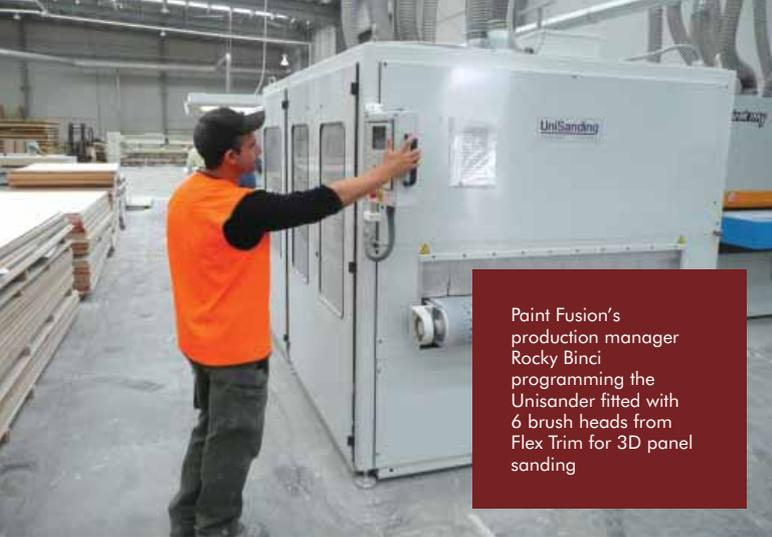
Paint Fusion's production manager Rocky Binci programming the Unisander fitted with 6 brush heads from Flex Trim for 3D panel sanding
